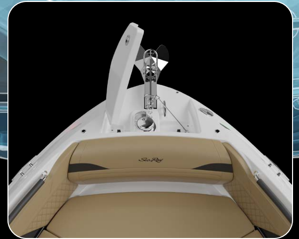
Windlass with rope and chain
